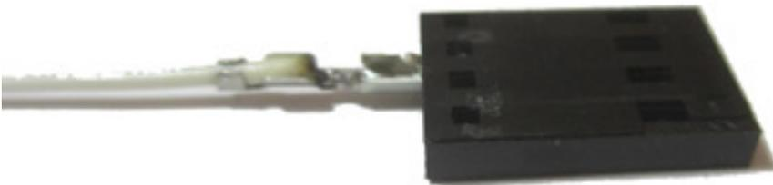
The pin is now properly placed inside the black housing. Note the tiny lever popping up through the opening when sliding in the pin.
