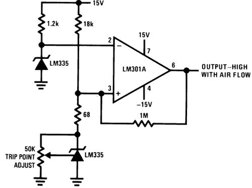
\*Self heating is used to detect air flow
