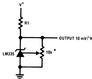
\*Calibrate for 2.982V at 25°C
