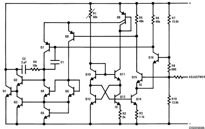
LM135/LM235/LM335, LM135A/LM235A/LM335A Precision Temperature Sensors
