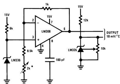
\*Adjust for 2.7315V at output of LM308
