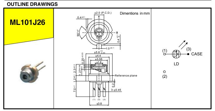
There is no model with a monitor photo diode in ML1XX26 series.
