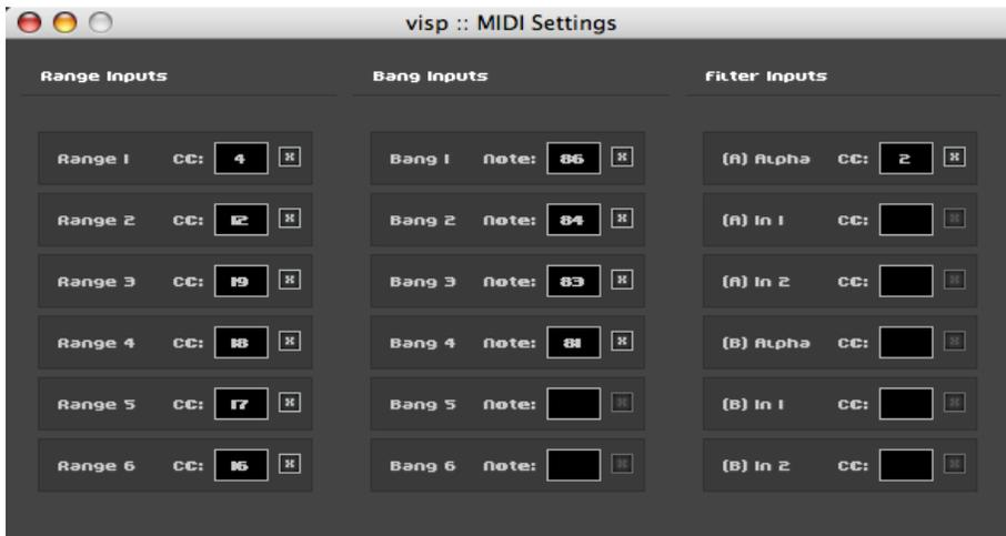
visp uses a simple 'MIDI Learn system'. Click on the "Range 1" field. This field should now be highlighted by a red box. Turn the I-CubeX Turn sensor. If everything is working, you should see the number box in the "Range 1" field change values to the corresponding Control Change number assigned to the Turn sensor in the I-CubeX editor. Close the MIDI settings window. Now, when you use the Turn sensor, you should see the "R1" slider move correspondingly.
